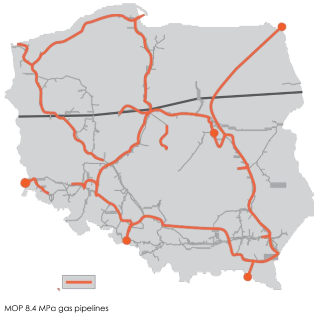
Figure 14: Expansion of the MOP 8.4 MPa system in 2009–2023.
